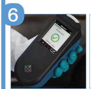
Measure 5 times by moving the Spectro, maintaining the vertical orientation
