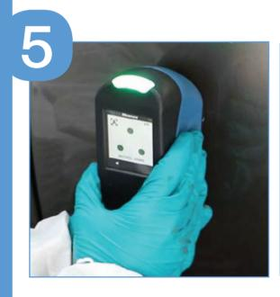
Position and hold the spectro on the prepared area. When all 3 LED's are green, press the measure button or simply tap the screen.
