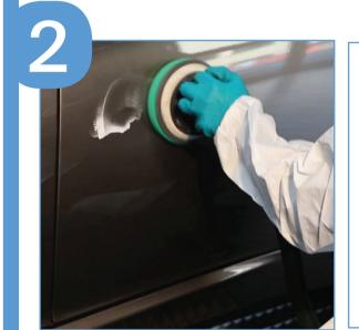
Prepare the measurement area by cleaning and then polishing
