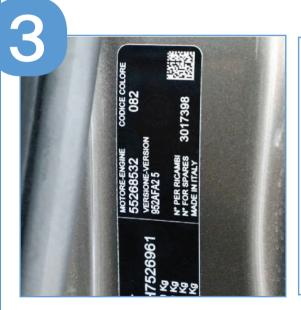
Locate and record the Colour Code of the vehicle
