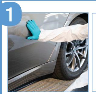
Identify an area close to the repair, free of scratches and as flat as possible
